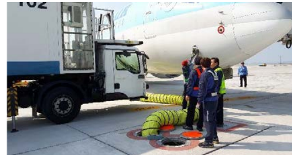
PC-Air in Incheon International Airport Terminal 2
