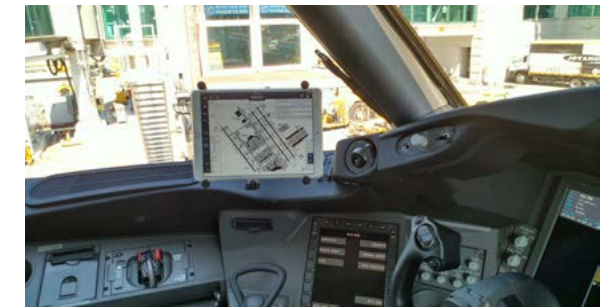
Cockpit equipped with portable EFB (Boeing 787)
